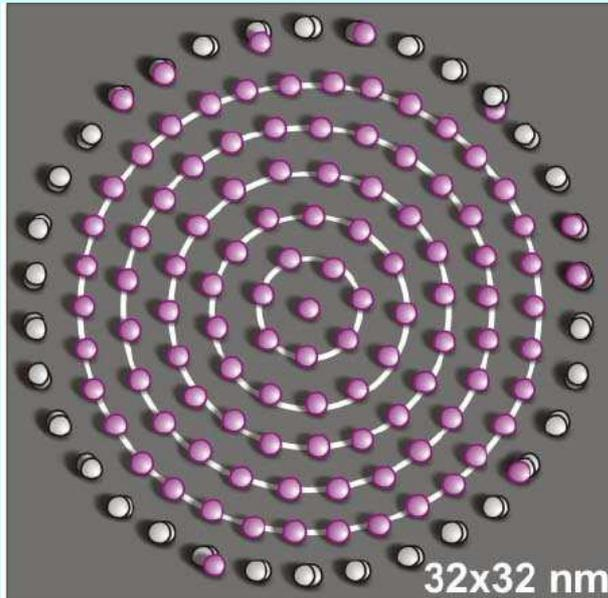
can be used to study these nanometer scale structures with atomic resolution in space and better than meV (micro electron Volt) resolution in energy. The data of the STM can be rendered in false color to produce breathtaking images that reveal standing wave patterns of coherent electrons inside the corrals. The presence or absence of a quantum mirage might be used to represent one bit of data in a region far smaller than any current electronic de-
