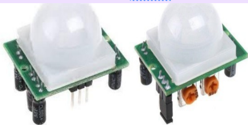
Figure.2 Motion detector module uses a motion detector IC and PCB mounted Fresnel lens
