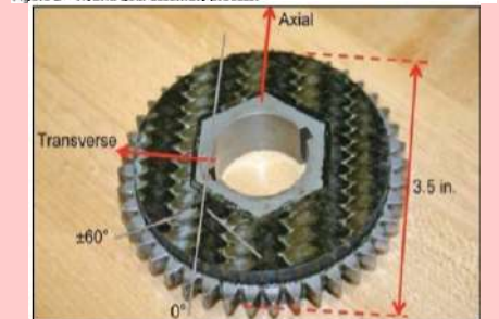
Figure 3. Assembled and cured hybrid gear.
